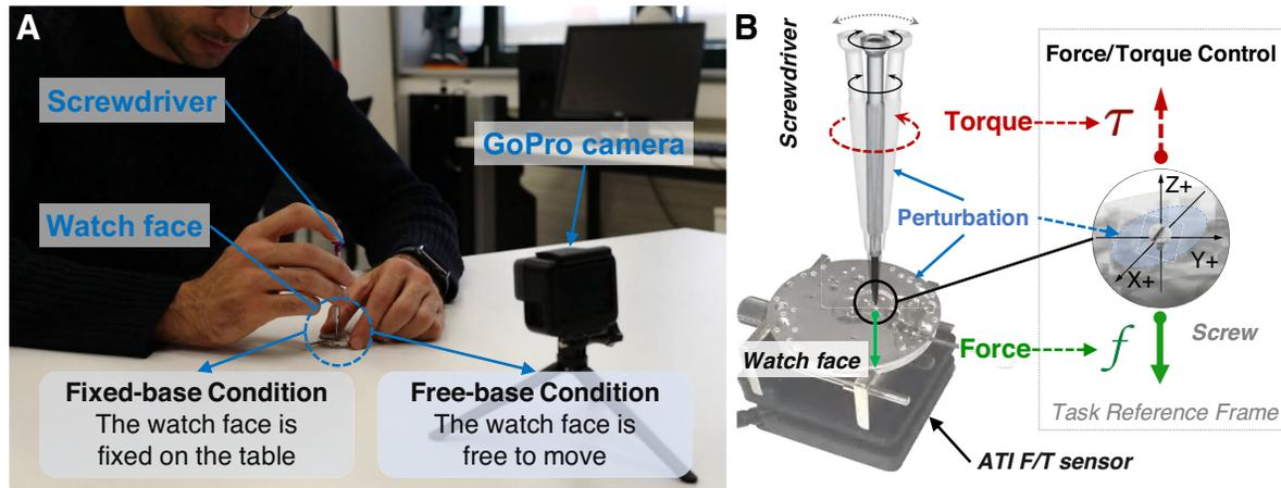
**Figure 1.** Experimental setup and apparatus. *A*: one GoPro camera was placed in front of the subjects to record hand movements while they performed the task. *B*: original watch face as used for the experiment. In the ex post facto experiments for analyzing hand poses, an ATI F/T (Force/Torque) sensor was mounted underneath the watch face to measure the applied resultant force and torque.
